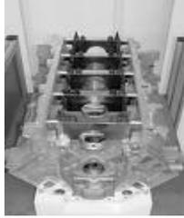
**Crankcase :** It may be cast integral with the cylinder
