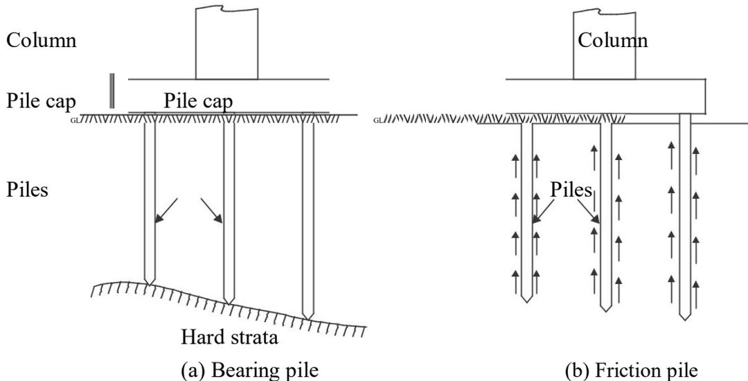
Fig. 2.2.4.1 Pile foundations
