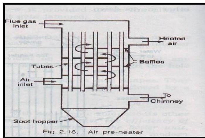
Hot flue gases pass through the tubes of air preheater after leaving the boiler or economiser.
