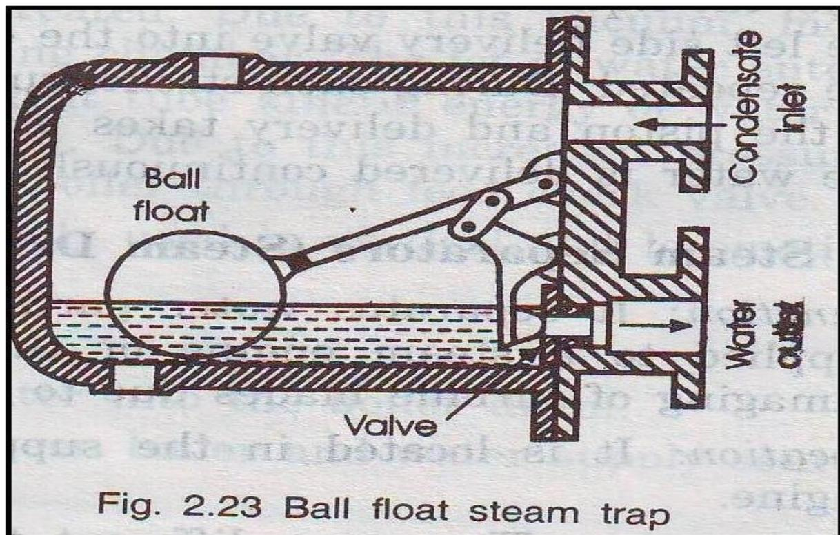
The condensed water enters the steam trap by gravity. When the water level in the trap rises high enough, the ball float is lifted. This causes the valve to open and the water is discharged through the outlet. After the discharge of water, the float moves down. This causes the valve to close again.
