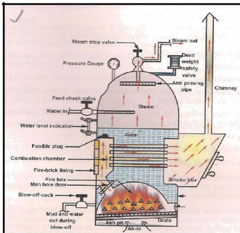
Coal is fed into the grate through the fire hole and burnt.
