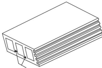
(e) **Sewer Bricks:** These bricks are used for the construction of sewer lines. They are manufactured from surface clay, fire clay shale or with the combination of these. They are manufactured in the sizes  $190 \times 90 \times 90$  mm and  $190 \times 90 \times 40$  mm. The average strength of these bricks should be a minimum of  $17.5 \text{ N/mm}^2$ . The water absorption should not be more than 10 per cent.
