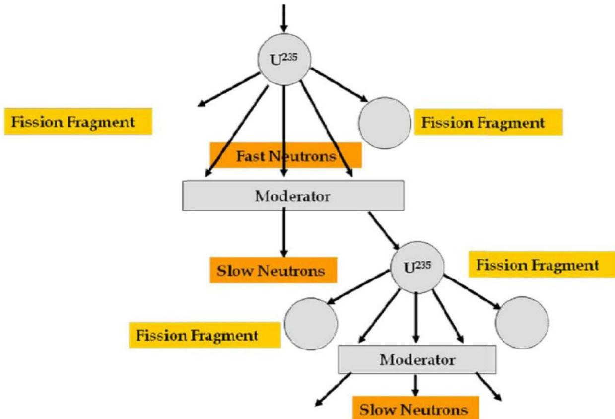
It is a process of splitting up of nucleus of fissionable material like uranium into two or more fragments with release of enormous amount of energy.
