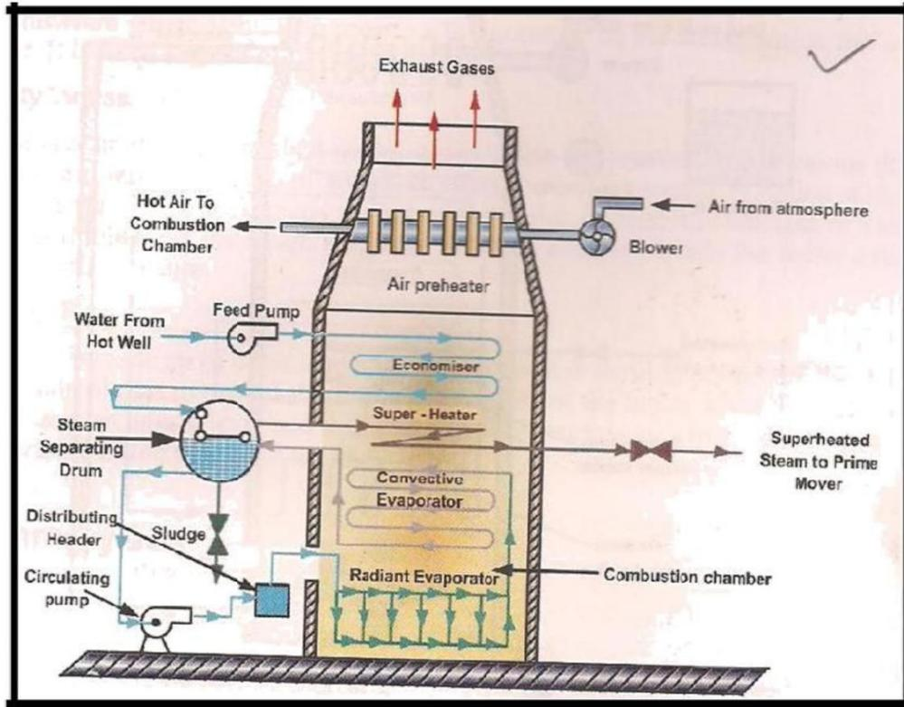
It is a water tube, forced circulation and externally fired high pressure boiler.
