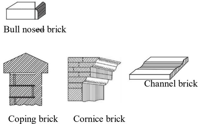
Fig. 1.1.11 Special shaped bricks
