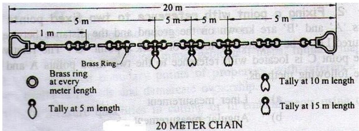
The chain is made of mild steel. The ends of the chain are provided with brass handles for dragging the chain on the ground. The outside of the handle is the zero point or the end point of the chain and the length of the chain measured from the outside of one handle to the outside of the other. The length of a link is the distance between the centers of the two consecutive middle rings.
