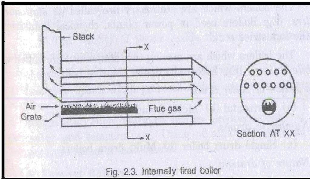
Fig. 2.3. Internally fired boiler
