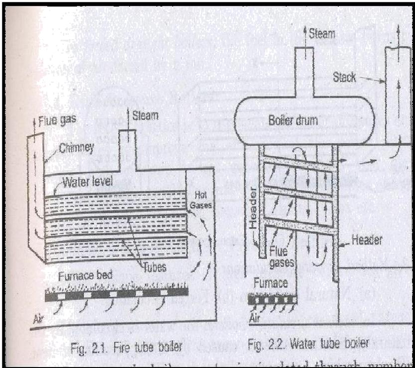
Fig. 2.1. Fire tube boiler
