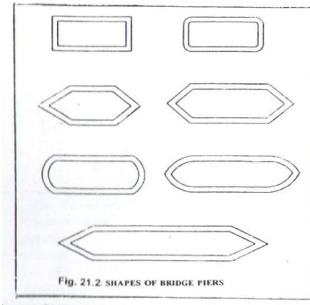
**b. Piers :** Piers are the intermediate supports for the superstructure. Piers transmit the loads from the superstructure of the bridge to the foundations. A pier essentially consists of a column or shaft and a foundation. They may have different configurations as shown in figure. These piers may be constructed with stone masonry or concrete.
