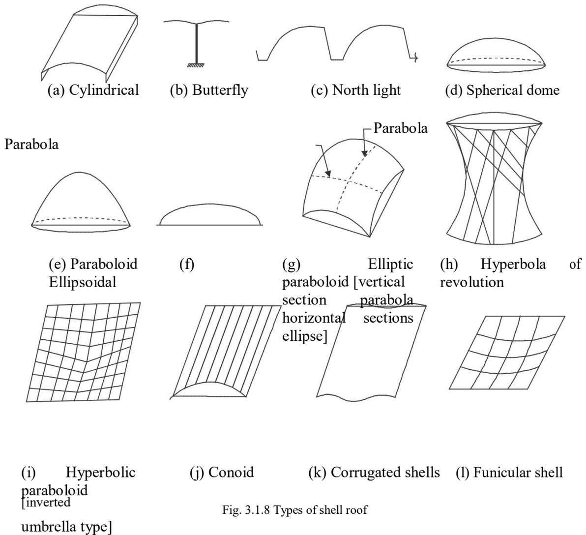
Fig. 3.1.8 Types of shell roof
