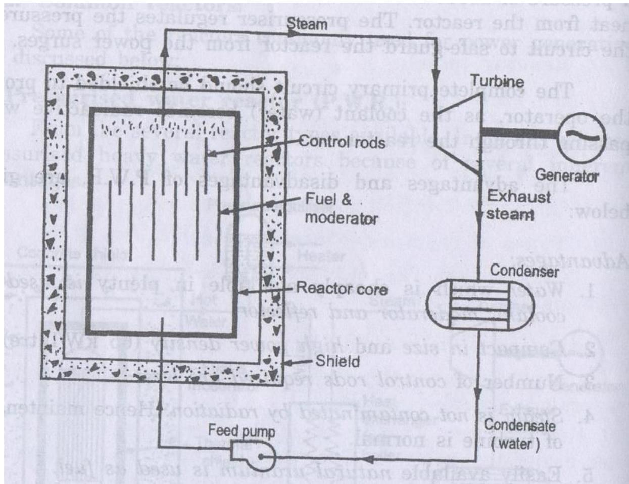
Nuclear power plant uses nuclear energy from radioactive element for generating electrical energy.
